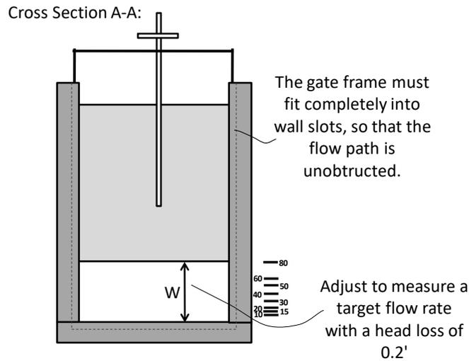
**Figure 32. End view of upstream gate of CHO**
