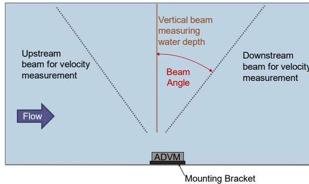
**Figure 35. Beam angle relative to flow path**
