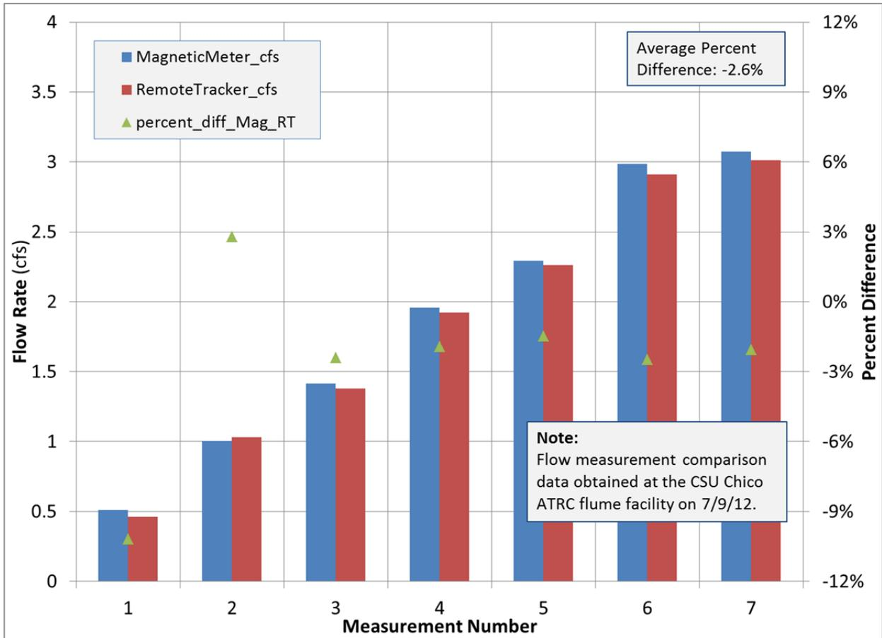
**Figure 6. RemoteTracker and CSUC ATRC Magmeter Comparisons**
