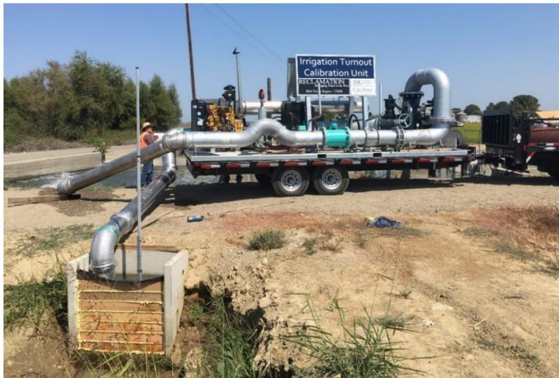
**Figure 13. USBR/ITRC Irrigation Turnout Calibration Unit**
