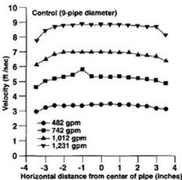
Fig. 1. Water velocity profiles under control conditions.
