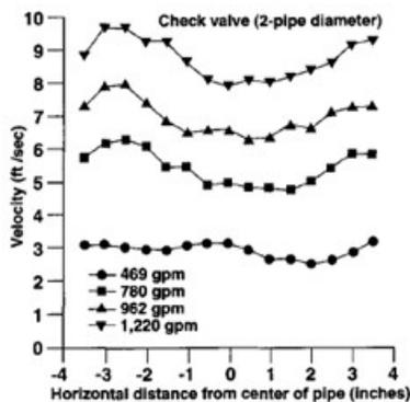
Fig. 2. Water velocity profiles under a check valve.
