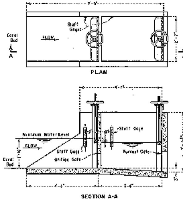
Figure 29. Schematic of a USBR CHO (from USBR, 2001)
