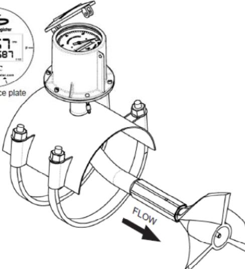
McCrometer will also mount a reverse-facing propeller on a standard open flow meter, which can be mounted on stands above low pressure pipelines.
