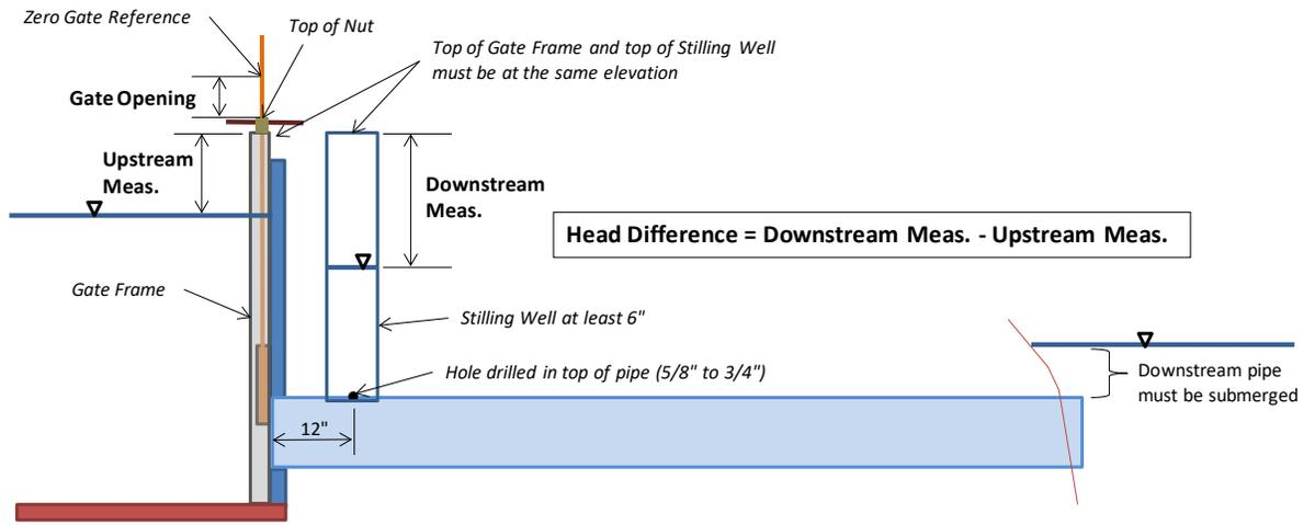
**Figure 14. Proper metergate dimensions – but lacking precast design.**
